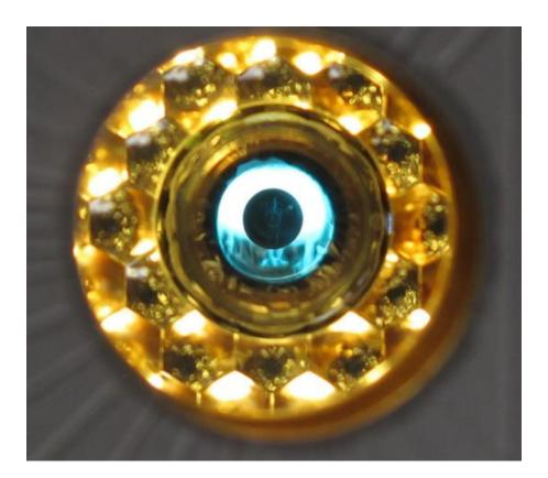
A photo of one of the targets used at the National Ignition Facility. The spherical capsule where thermonuclear fuel is loaded can be seen in the middle.
