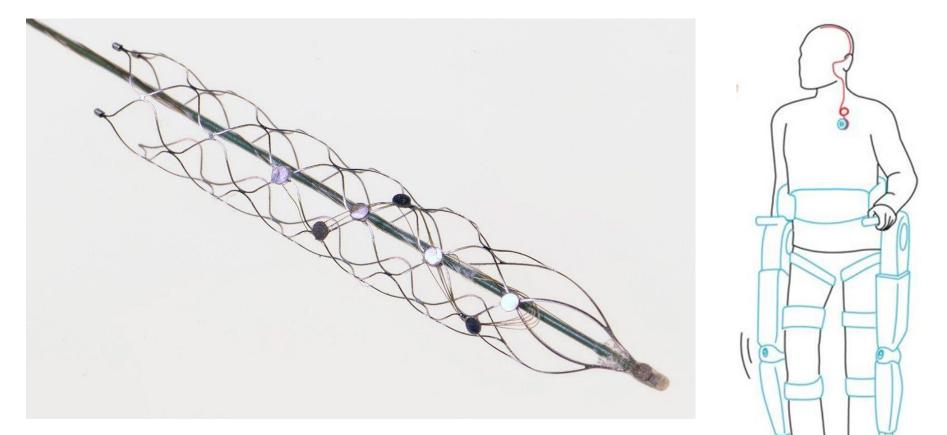
DARPA's Reliable Neural-Interface Technology (RE-NET) program A paralyzed man has walked again thanks to a braincontrolled exoskeleton with two implants, each containing 64 electrodes, on the parts of his brain
